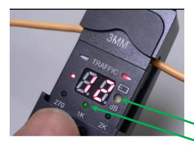
Battery Level LED LED Indicates a 1kHz Tone
